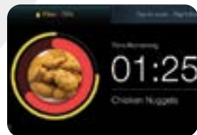
Red ring indicates cook time progress; gold ring indicates remaining oil life to filter
